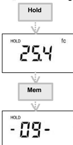
The measurement value to be memorized is locked by the **Hold** key in the display. By pressing the key **Mem** you will enter the value to be stored in the next free memory location.
